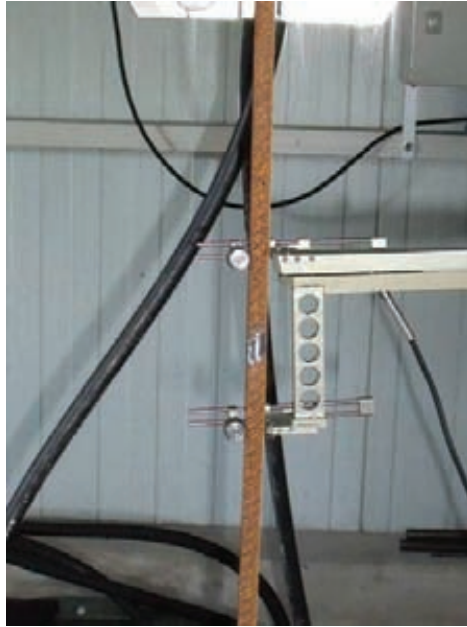
Fig. 13 One of the bars placed in the compression machine
