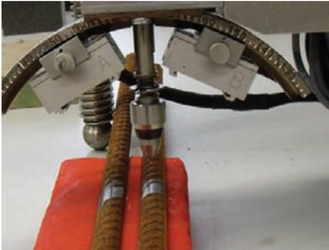
Fig. 11 Sight of the calibration process before loading the bars
