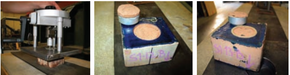
Fig. 8: Pull-off test ready to be executed on a strengthened half-brick, and some typical failures (within the brick and at the brick-resin interface) (Panizza et al. 2009).
