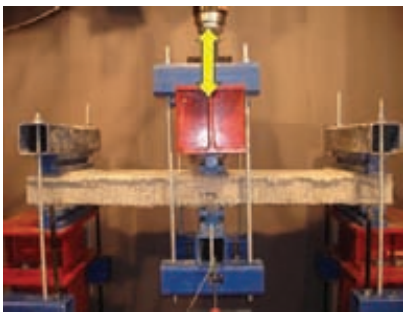
Fig. 3 Out-of-plane loading: (a) Test set-up; (b) Actuator displacement history.
