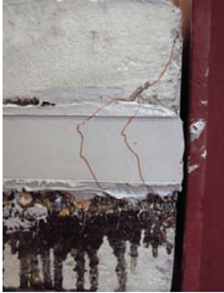
Figure 16. Localization of crack. Failure cone for pull shear test.
