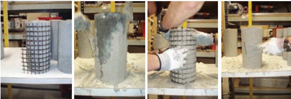
Fig. 10. Concrete confinement procedure
