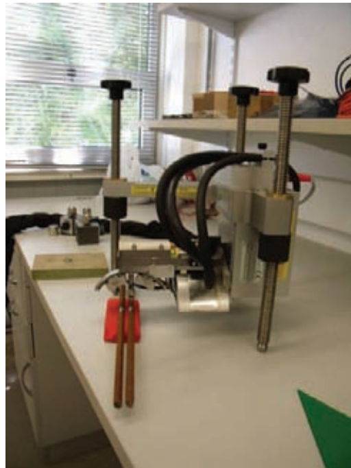
Fig. 11 The detection unit of the equipment on the two corrugated steel bars
