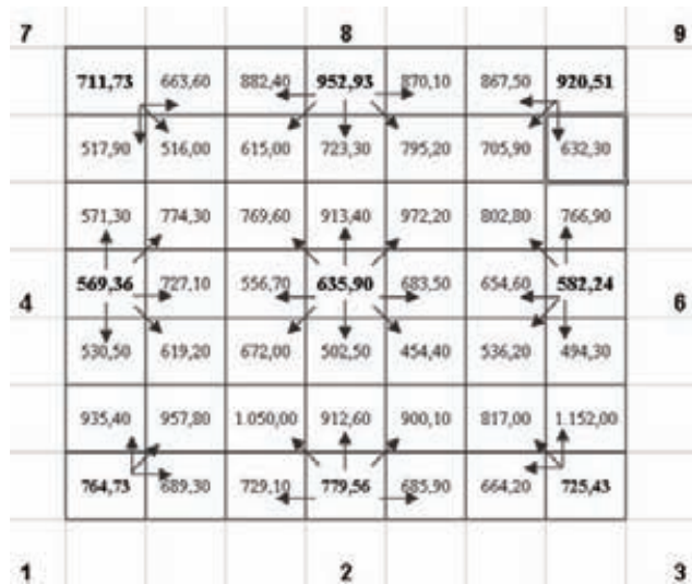
Fig.9 Velocity distribution. Cavity wall. Case study A.
